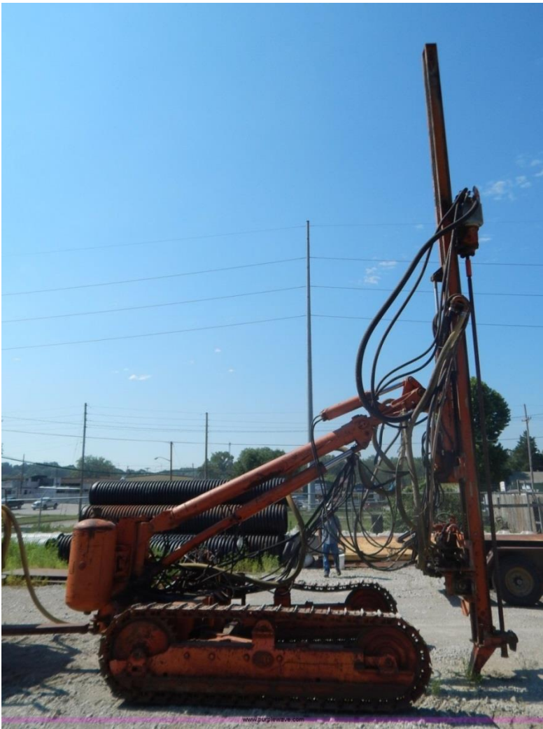
Typical Air Track Rock Drill, drilled a 3" dia. hole
