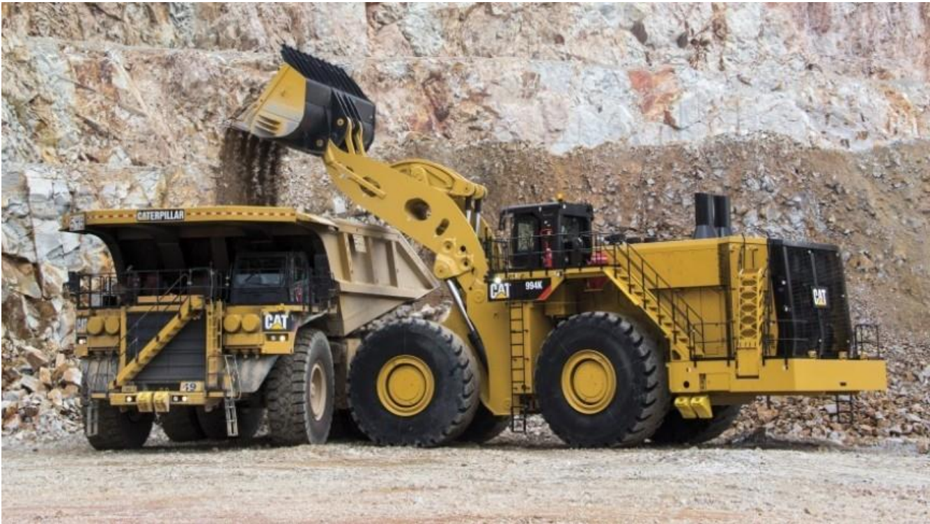
A 992 Caterpillar 10 cy front end loader, loading a 50 ton rock truck
