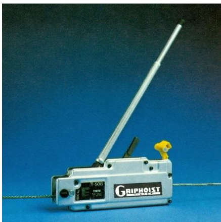
Griphoist, 8,000 lbs. pulling capacity for tensioning the unloaded gut line to about a 25' sag.
