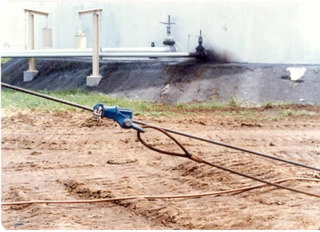
Sauerman Continuous Cable Clamp. Safe Working Load same as the gut line. Used as a safety with the sling hooked to the T-bar anchor at the canyon bottom.
